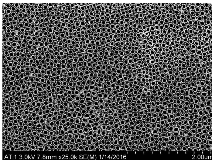
This scanning electron microscope image shows a titanium sample anodized with 1% hydrofluoric acid for 10 minutes at 20 V. After anodization, the titanium surface showed nanotubular-like structures with an inner diameter of ~80 nm. (Image courtesy of Luting Liu, Webster Nanomedicine Lab at Northeastern University)
