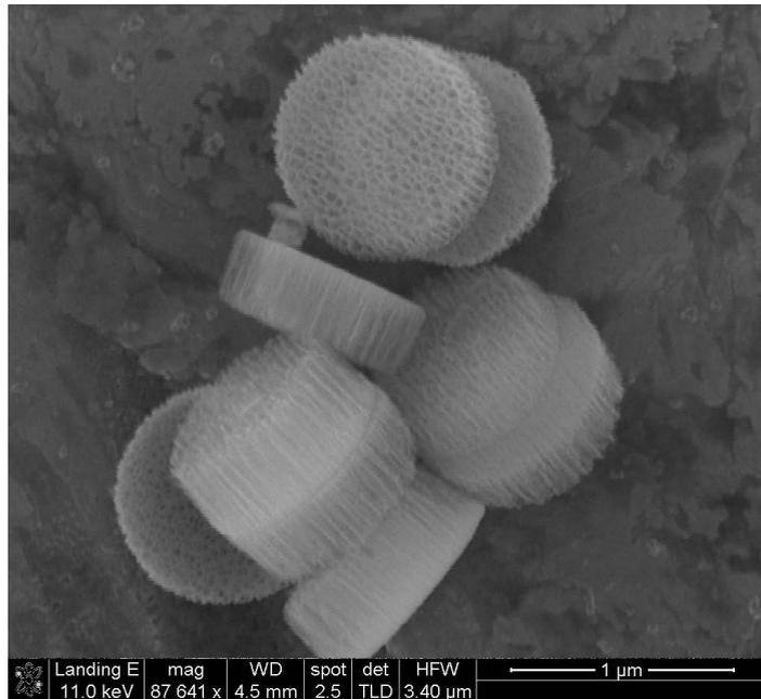
This scanning electron microscopy image shows multistage vectors (MSV) produced at the Houston Methodist Research Institute. Each MSV measures 1 μm wide and 400 nm high. Nanoparticles containing microRNAs fit inside the 40-to-80-μm MSV pores. (Image courtesy of Dr. Haifa Shen, Houston Methodist Research Institute)
