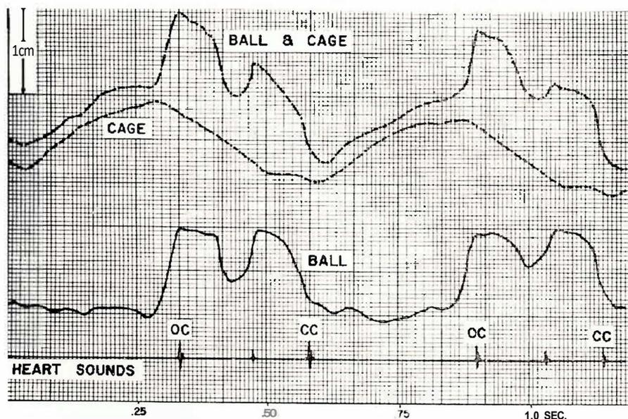
**Figure 3.** Displacement time curve of mitral ball and cage traced frame by frame from cine film with heart sounds superimposed. Bottom trace represents ball motion alone, using base of cage as a fixed reference point. OC = opening click. CC = closing click.
