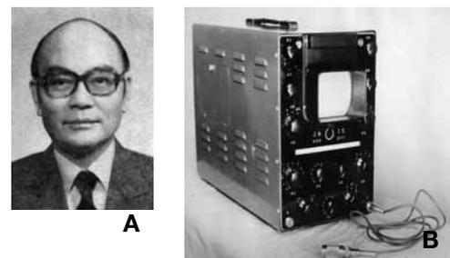
Figure 2. (A) Shih An (courtesy XF Wang) and (B) China’s earliest ultrasonic diagnostic device, the A-mode scanner, made in Jiangnan Shipyard in Shanghai and used in 1958 by An for diagnosing various diseases in patients at the Shanghai Sixth People’s Hospital (courtesy B Hu and XF Wang).
