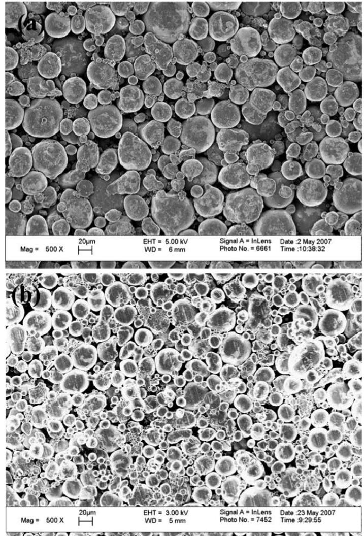
**Figure 1.** Scanning electron microscopy images of nickel-titanium alloy (NiTi) surfaces. (a) Microstructured NiTi, Mag 500x, bar = 20  $\mu\text{m}$ . (b) Submicrostructured Nitinol, Mag 500x, bar = 20  $\mu\text{m}$ <sup>22</sup>
