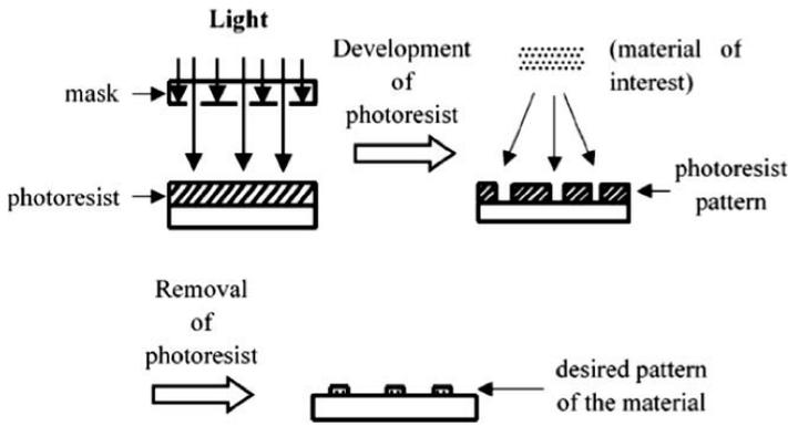
**Figure 3.** Schematic of micro/nanopatterning by photolithography.<sup>44</sup>
