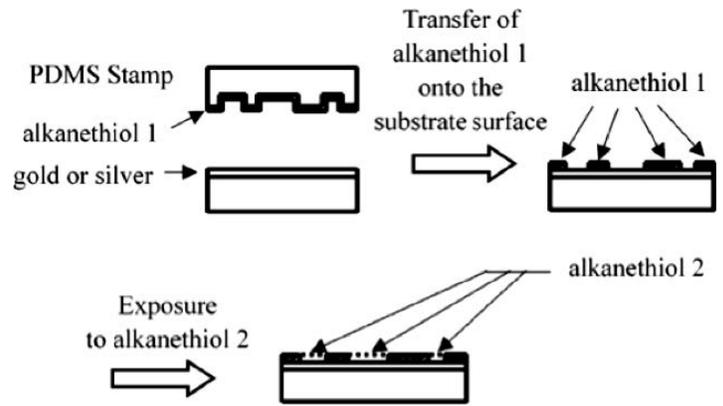
**Figure 4.** Schematic of micro/nanopatterning by microcontact printing.<sup>44</sup>
